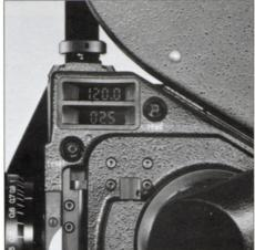
film is shown in meter of feet on a scale on the magazine. It is governed by an arm on the film roll. The camera also possesses a visual sync control red lamp in the viewfinder image. Variable frame speeds are also shown in the viewfinder image with a green control lamp.
