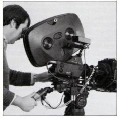
with the ARRIFLEX bridge plate for all 35 mm and all 16 mm ARRIFLEX cameras. It is easily and quickly fitted and the camera assistant has the choice of operating it from the right or left hand side. One of the advantages of the system is that it permits easy remote control with follow focusing by means of a flexible shaft. The marking discs can be exchanged.
